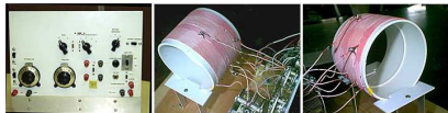
Fig. 1 - Single-Tuned Four-Band Crystal Radio Set, Version 'C'. These are actually pictures of Version B as described in Article #22, converted to version C, as described in this Article, but modified with the
